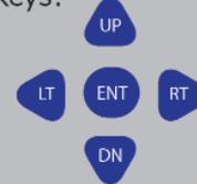
Up and Down: to navigate or adjust a menu parameter
