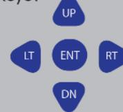
Up and Down: to navigate or adjust a menu parameter
