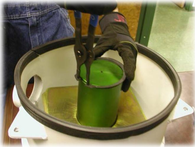
7. Line up the tabs with the lid. Secure the handles.
