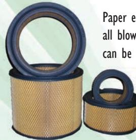
Paper elements are the recommended media for all blower applications since PD blower tolerances can be as small as 0.001 inches. The paper filter media has an efficiency of 99% on 1 micron particles compared to competing polyester elements at 10+ micron particles.
