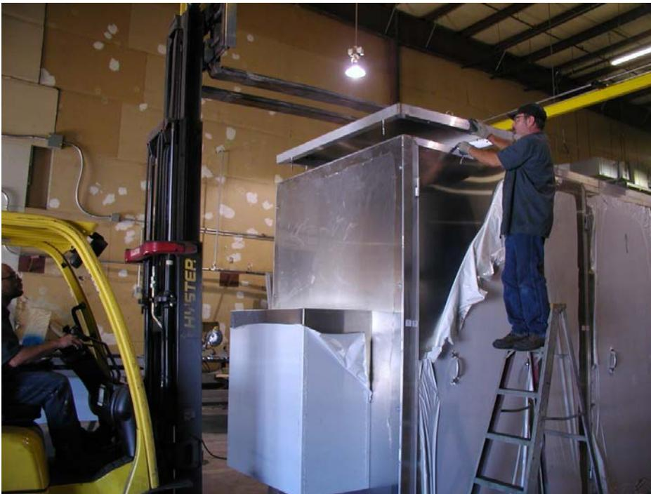
9. If necessary, install the doors. Depending on what type of hinge you have, you may have to fasten the bolts. Welded hinges allow for the door to lift off and on.
