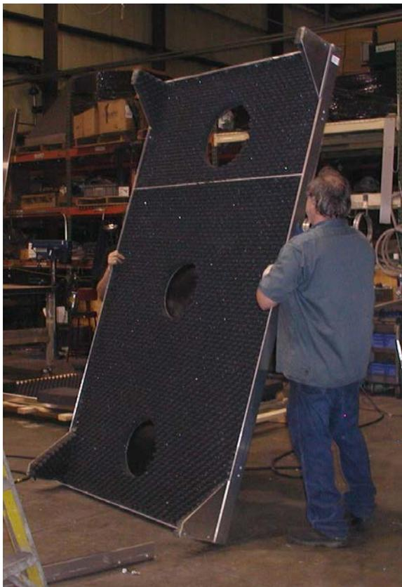
2. Use (2) 3/8 bolts and washers on each side to fasten the Spars to the End Panel.
