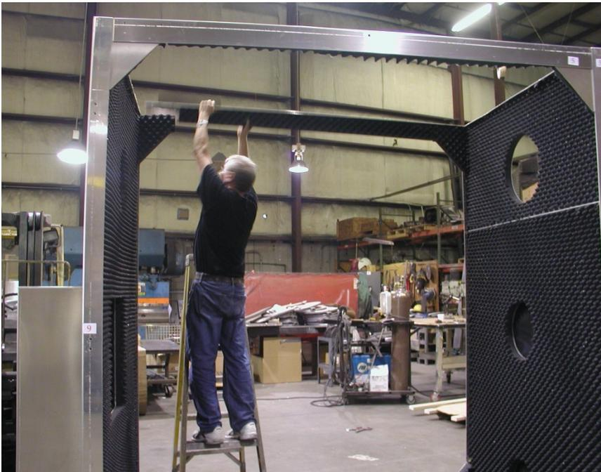
7. Use (4) clamps to temporarily secure the Top Spars to the End Panels. See below.
