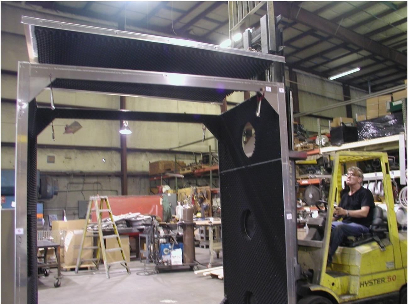
10. Use 3/8 Bolts to fasten the Roof Panel to the Top Spars.
